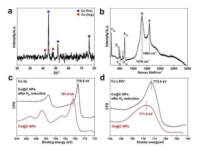
**Fig. 2.** Structure characterizations of Co@C NPs. (a) XRD pattern of fresh Co@C NPs, (b) Raman spectrum of Co@C NPs, XPS spectra of Co 2p region (c) and Co L3VV Auger spectra (d) of the fresh Co@C NPs and the sample after *ex situ* reduction by 7 bar of  $H_2$  at 120 °C.
