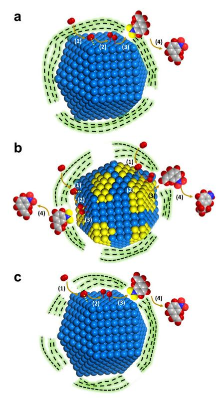
**Fig. 5.** Proposed reaction pathways of hydrogenation of 3-nitrostyrene on Co@C NPs with coverage of carbon layers (a) and defective coverage of carbon layers (b). In schematic illustration **Fig. 5a**, the chemoselective hydrogenation of  $-NO_2$  groups can be divided into the following steps: the diffusion
