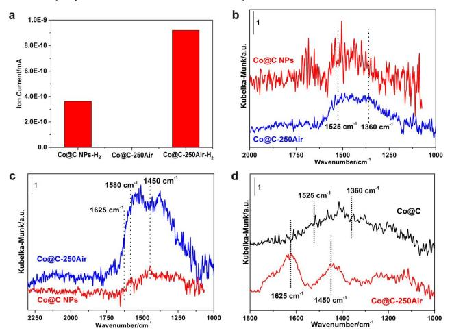
**Fig. 4.**  $H_2$ - $D_2$  exchange and DRIFTS adsorption experiments. (a) Enhancement of the ion current in mass signal of HD during the  $H_2$ - $D_2$  exchange experiment over Co@C- $H_2$ , Co@C-250Air and
