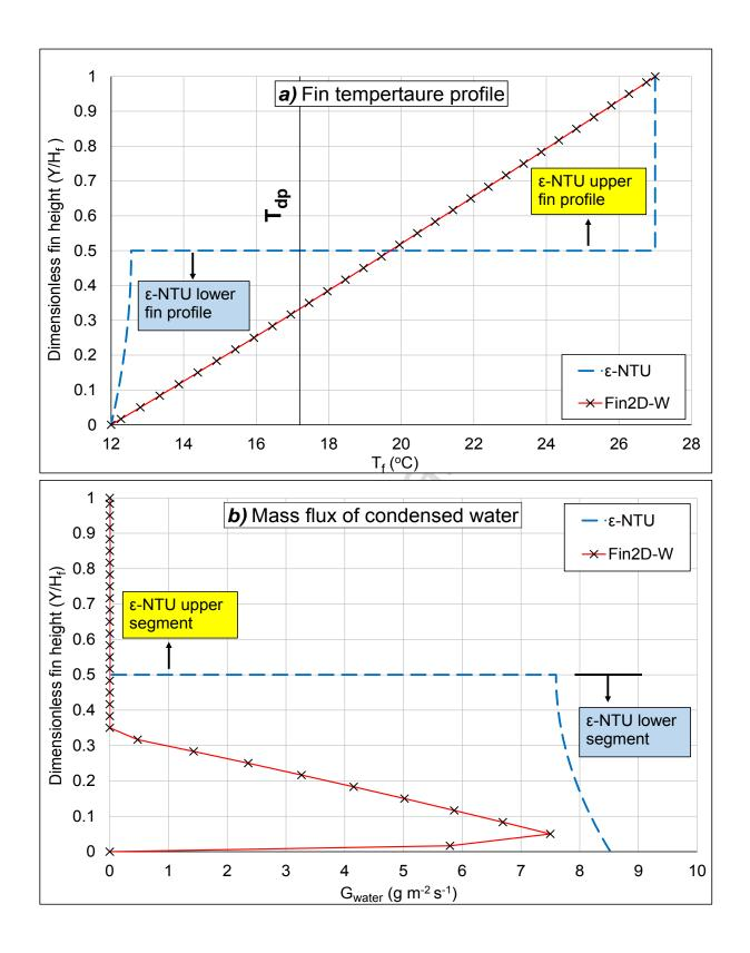
Fig. 8 – (a) Fin temperature profile and (b) mass flux of condensed water, at half the fin depth, for a point in R3. This represents Case II, when  $T_{lt} = 12.0$  °C and SH=15.0 K.
