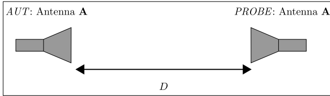
Figure 6.10: Measurement set-up for the case of two identical antennas (Measurement M ).
