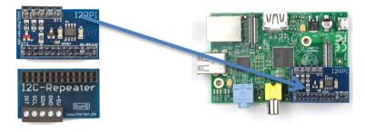
Fig. 2. I2C Interface for the GPIO
