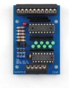
Fig. 3. Digital input card 8 bit
