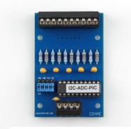
Fig. 5. Analogue input card 12 bit
