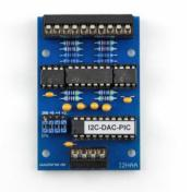
Fig. 6. Analogue output card 12 bit
