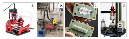
Figure 2. Microprojects' DIY-DkM: a. bq Cyclone (bq, 2016), b. Graber i3, c. Injected pieces and its printed mould (Stratasys, 2015), d. PIM-Model-20A of LNS Technologies, to convert a driller press into a plastic injection machine (LNS-Technologies, 2015).
