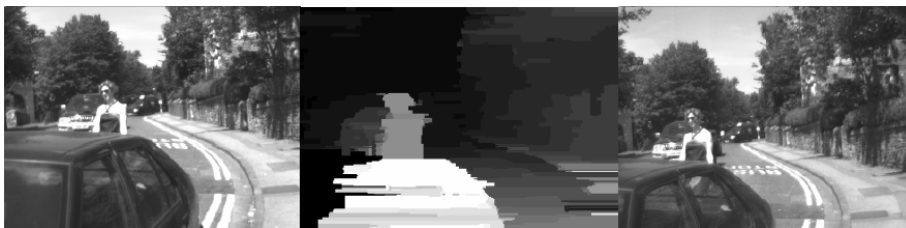
Figure 2.12 Depth map extraction from stereo images either side
