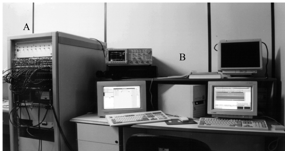
Figure 2.20 Sound generation and processing system. A represents the Huron system based on 40 analogical outputs and 8 analogical inputs and 8 DSPs 56002. The system was used for HRTFs measurements and experiments for mono and multi sources localization. B represents the computer where the HRTF's were processed and off-line processing of the spatialized sounds performed.
