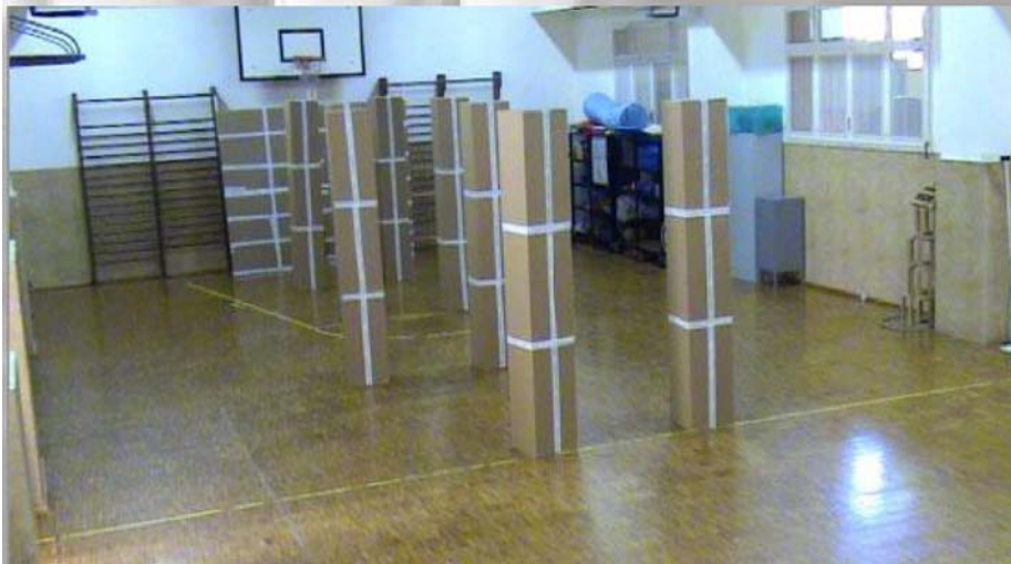
Figure 5.15 The real scenario of the experiment. The scenario was located in a hall of 258\text{m}^2 . The trajectory is created by soft-box carton columns; a square made by carton boxes placed at the hall background was used as a wall.
