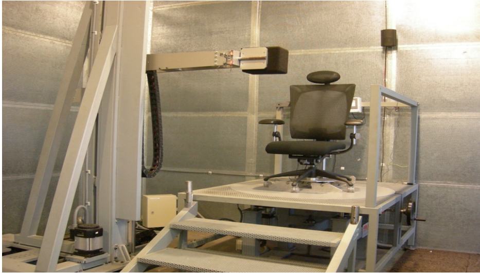
Figure 2.19 The anechoic chamber with small reverberation level and the robotic system. The walls and floor of the chamber are lined with sound absorbing wedges. The whole robotic system can be moved to place the loudspeaker at any location in radius of 5 meters. A chair for manikin is represented in a fixed platform.
