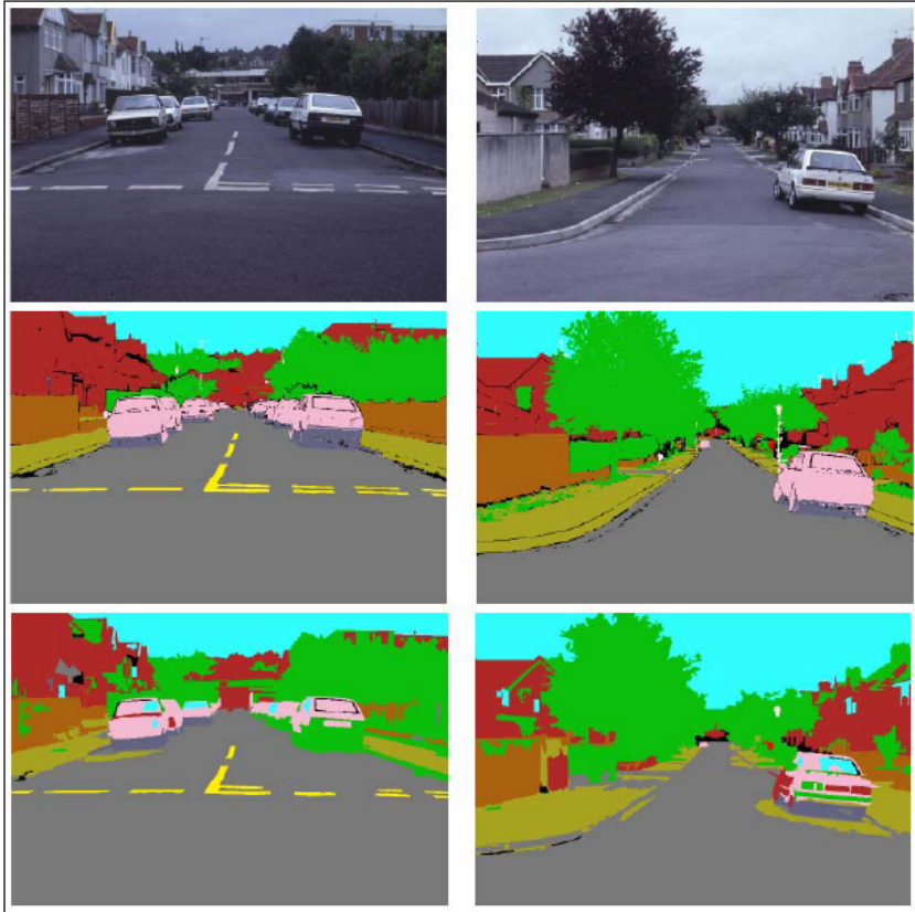
Figure 2.10 Example of image segmentation. Each column represents the segmentation of two different images
