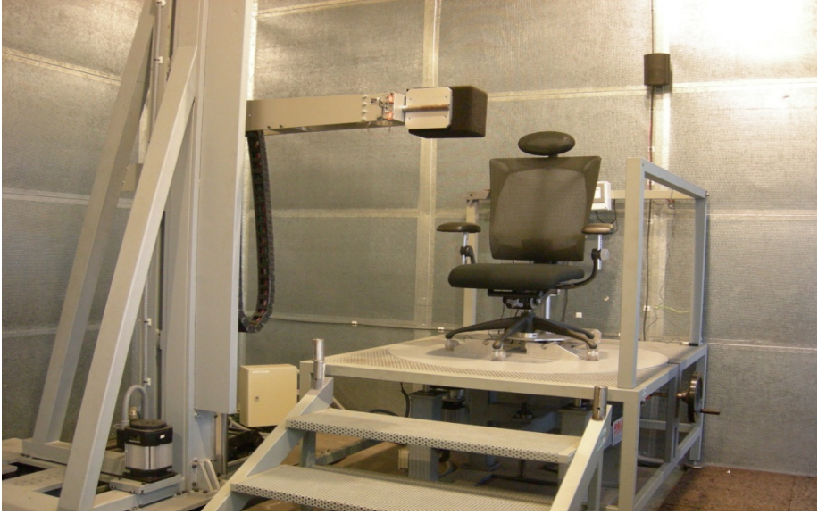
Figure 4.6 The anechoic chamber. The walls and floor of the chamber are lined with sound absorbing wedges. The whole robotic system can be moved to place the loudspeaker at any location in radius of 5 meters. A chair for manikin is fixed in a platform.
