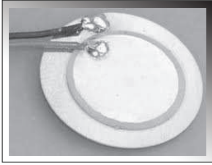
Fig. 1 Piezoelectric sensor with electrodes and electrical connection
