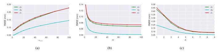
Figure 6: Evolution of the RMSE values of the ET models with the different hyperparameters for the three displacement coordinates using the 70%/30% data splitting approach: (a) the minimum number of samples to split a node  $(n_{min})$ , (b) the number of trees in the ensemble (M) and (c) the number of input variables randomly selected at each node (K).
