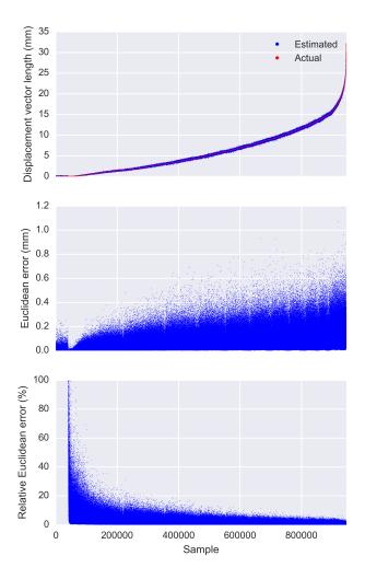
Figure 10: Performance assessment results with samples ordered according to the actual displacement vector length using the best model for the data splitting approach leaving one liver for test, including the estimated and the actual displacement vector lengths for all the samples (*top*), the Euclidean error for all the samples (*middle*) and the relative Euclidean error for all the samples (*bottom*).
