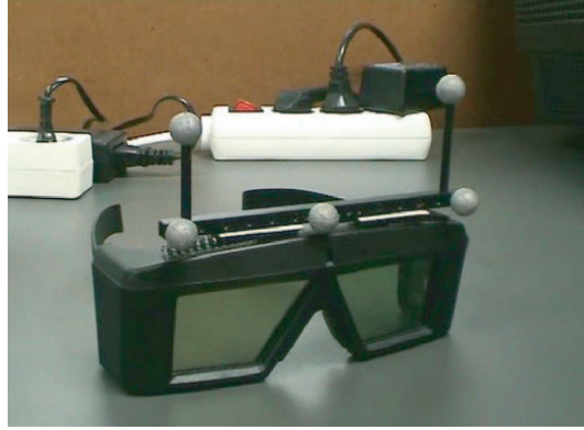
Figure 4.2: Image of the shutter glasses (CrystalEyes3, Real D, StereoGraphics, Beverly Hills, USA) used to visualize the VE inside the CAVE. Reflective targets are attached to them in order to detect their position and orientation while the subject navigates in the VE.
