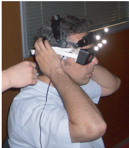
Figure 4.6: User with TCD probes and shutter glasses for visualizing VE with stereoscopy.
