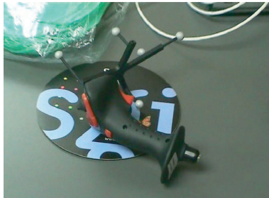
Figure 4.3: Image of the wireless joystick (Flystick, Advance Realtime Tracking GmbH, Weilheim, Germany) used to navigate. Reflective targets are attached to it in order to detect its position and orientation while the subject navigates in the VE.
