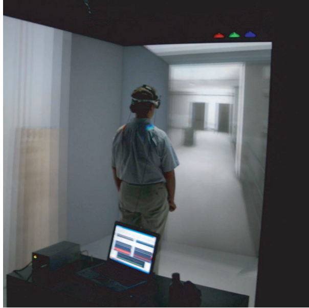
Figure 4.10: User visualizing the automatic navigation in the Reality Center. The probes are placed on the user's head and connected to the Doppler Box, which is connected to a PC that runs QL software.
