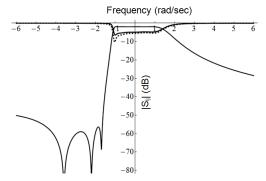
Fig. 2. Target S-parameters for an asymmetrical lossy filter (low-pass prototype with unity source and load resistances) [p. 60 in 20]: solid lines for  $|S_{21}|$  and  $|S_{11}|$ ; dashed line for  $|S_{22}|$ .
