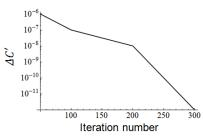
Fig. 10. Cost function associated with the extended coupling matrix from Table VIII, calculated using (15) using the Nelder Mead algorithm. Using (15) we reach a solution while using (13) we fail.
