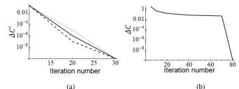
Fig. 8. Cost functions associated with the extended coupling matrix from: (a) Table VI; and (b) Table VII. (solid line- Nelder Mead, dashed- Simulated Annealing, dots-Differential Evolution)
