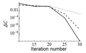
Fig. 4. Cost function associated with the extended coupling matrix from Table II, calculated using (16). (solid line- Nelder Mead, dashed- Simulated Annealing, dots-Differential Evolution)
