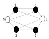
Fig. 9. Parallel coupled filter topology
