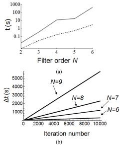
Fig. 1. Computation gain using *Mathematica 9.0* with an Intel i7 processor and 2 GB RAM: (a) Time taken *t* for solving (12) (solid lines) and (14) (dashed line) for arbitrary 2nd to 6th order filters with symmetrical N+2 order coupling matrix (using symbolic non-numerical coefficients); (b) Results against iteration number for different order coupling matrices (using numerical coefficients) (with the cost functions  $\Delta C$  and  $\Delta C'$  giving the same final results).
