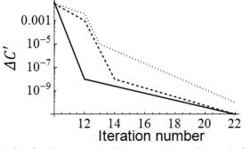
Fig. 5. Cost function associated with the extended coupling matrix from Table III, calculated using (15). (solid line- Nelder Mead, dashed- Simulated Annealing, dots-Differential Evolution)
