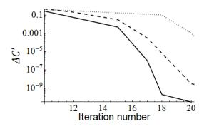
Fig. 3. Cost function associated with the extended coupling matrix from Table I, calculated using (15). (solid line- Nelder Mead, dashed- Simulated Annealing, dots-Differential Evolution)
