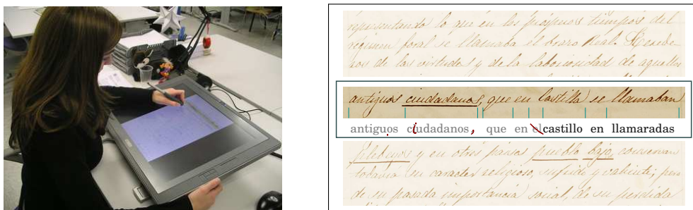
Figure 1.1: Left: illustration of CATTI multimodal user-interaction using a touch-screen. Right: page fragment showing a line image being processed, with a partially corrected system suggestion (in grey and black roman font) and the (previous) corrections made by the user through pen strokes and handwriting input marked in red.
