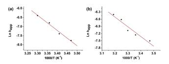
Fig. 3  $\ln k_{\rm app}$  vs. 1000/T plots for 4-NP (a) and NF (b). Volume of colloidal gold suspension of 25 µL
