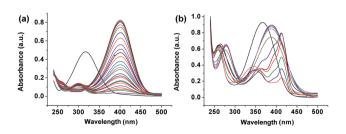
Fig. 2 Spectra of (a) 4-NP and (b) NF reduction catalysed by CB7-protected AuNPs. Black line:  $5.0\times10^{-5}$  M nitro compounds in water. Other lines are after the addition of  $100\times$  NaBH<sub>4</sub> and a volume of the catalyst suspension, 30  $\mu$ L for 4-NP and 25 for NF.
