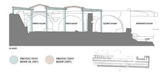
Figure 13: Protection roof sof the basilica, section.
