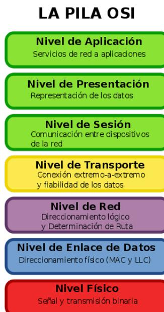
Figura 3.5 Pila OSI
