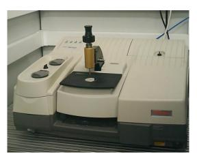
Figure 3.5. Thermo Nicolet 5700 FT-IR spectrometer
