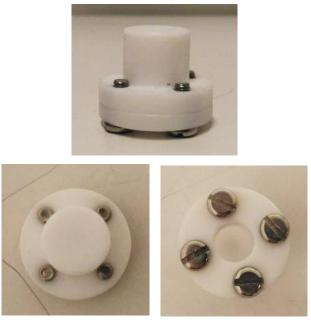
Figure 3.31. Pictures of the home-made gravimetric cell taken from three different views: front, top and bottom side
