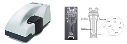
Figure 3.2. Zetasizer Nano ZS (Malvern) equipment and its Zetasizer nanocell
