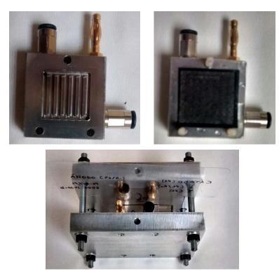
Figure 3.33. Pictures of the single DMFC used to evaluate the performance of the composites
