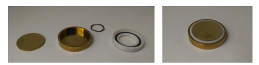
Figure 3.29. *BDS-1308* liquid parallel plate sample cell used for proton conductivity measurements
