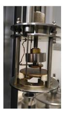
Figure 3.30. *BDS-1200 (Novocontrol)*, parallel plate capacitor cell used for the electrical conductivity measurements
