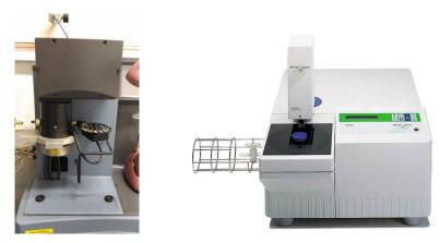
Figure 3.12. TA Instruments TGA Q-500 analyzer and Mettler-Toledo TGA/SDTA 851<sup>e</sup> modulus analyzer
