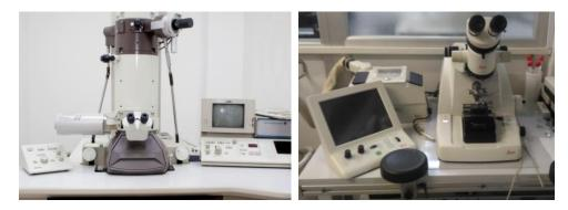
Figure 3.15. *JEOL JEM-1010* transmission electron microscope (left) and ultra-microtome *Leica EM UC6* (right)
