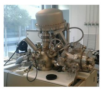
Figure 3.8. XPS SCALAB 210 multi-analysis system
