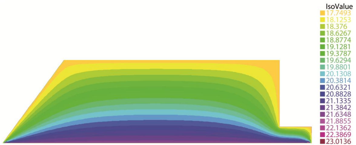
13. Results of the CFD simulation (horizontal section of the model) with air heating and no solar radiation: 30 December, 8:00 h.
