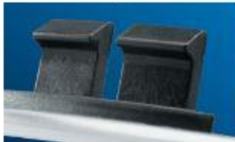
Close-up of automotive wheel cover snaps
