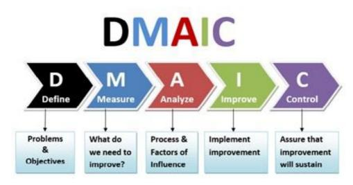
Figure 1.5. DMAIC – Six-Sigma Analysis
