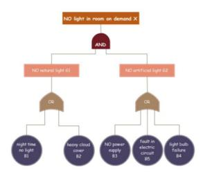
Figure 1.14. Fault Tree
