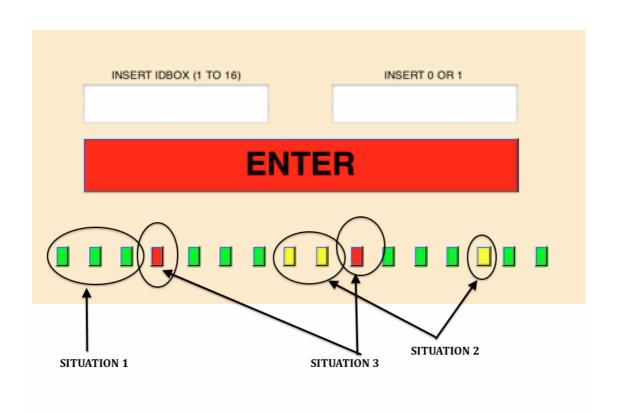
Figure 3.33. Alarm Levels in Interface
