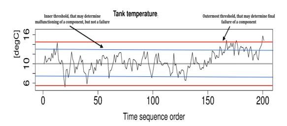
Figure 2.2. Process Monitoring
