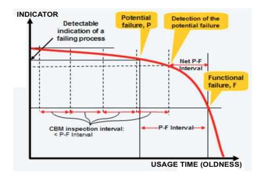
Figure 1.13. Condition Based Maintenance (CBM)
