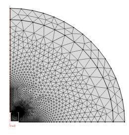
Figure 2: Mesh of the subwoofer's simulation model.
