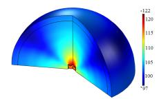
Figure 4: 3D Representation of Sound Pressure Field of a single subwoofer at frequency f=200 Hz.
