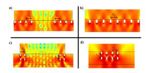
Figure 6: Scheme of the four configurations of subwoofer arrays. Detail of the Sound Pressure Level at f=200 Hz.
