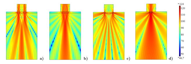
Figure 8: Simulation of four types of arrays. a) LR Parallel Array; b) Centered Parallel Array; c) LR Cardioid Array; d) Centered Cardioid Array.
