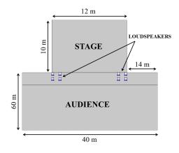
Figure 7: Location of the loudspeakers in the LR Cardioid Array simulation model.
