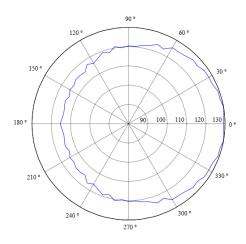
Figure 5: Radiation polar plot of a single subwoofer at f=200Hz.
