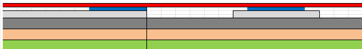
Fig. 5 - Position of track supports in separation between slab track (left) and ballast (right) track used for simulations in figures 6 and 7.
