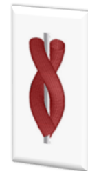
Figura 130: hilado conductor (filamento conductor exterior)
