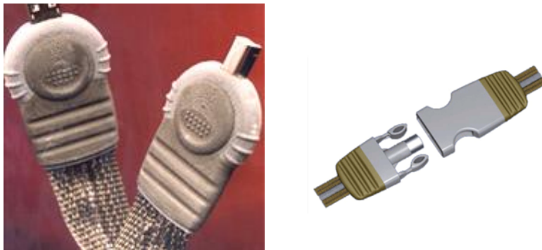
Figura I14. Conectores textiles: cable textil USB y hebillas [45]
