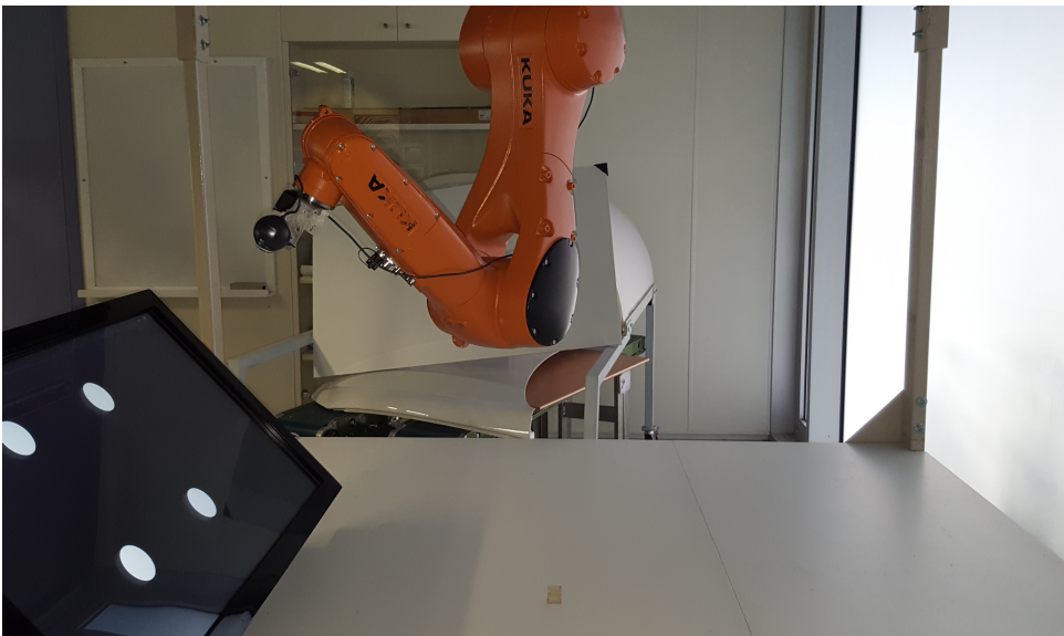
Figure 5.13: Experimental setup: 6R serial industrial manipulator in ceiling position with the camera rigidly attached to the robot end-effector (eye in hand configuration) and a screen to display the object markers.
