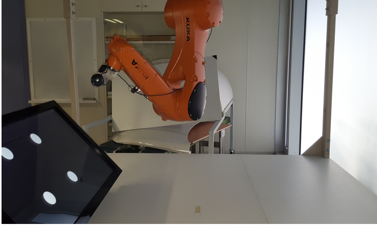
Figure 4.19: Experimental setup: 6R serial industrial manipulator in ceiling position with the camera rigidly attached to the robot end-effector (eye-in-hand) and a screen to display the object markers.
