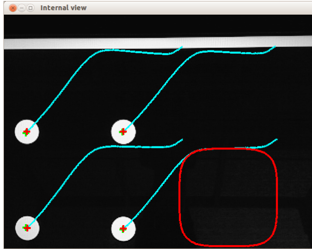
Figure 4.23: Image features trajectories for the visibility constraints experiment in IBVS with no errors in the gradient vector. Snapshot in the desired pose.
