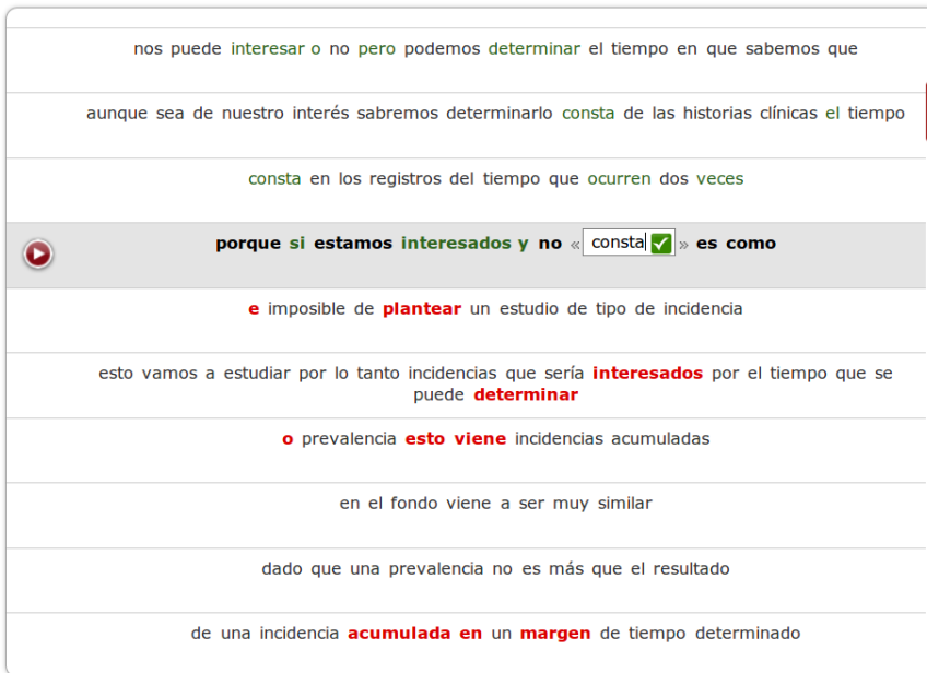
Figure 4.3: A screenshot of the transcription interface in intelligent interaction mode. Low-confidence words appear in red and reviewed low-confidence words in green. The word being edited in this example is opened for review, and the text box can be expanded to the left or right by clicking on << or >>, respectively. Clicking the green check button to the right of the text box confirms the word as correct.
