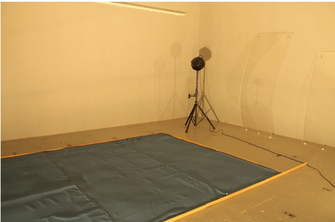
*Figure 12. Melamine Foam + Fabric set up*
