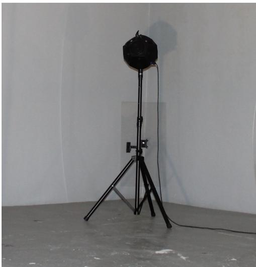
*c. Omnidirectional Loudspeaker*
