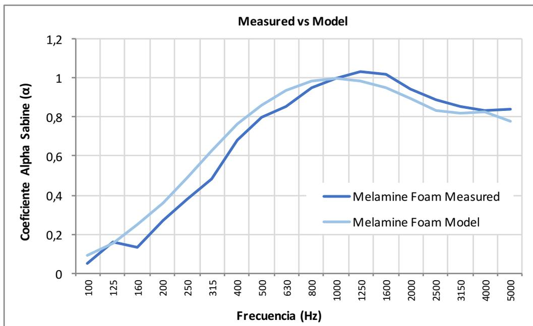
Figure 16. Absorption Coefficient Melamine Foam
