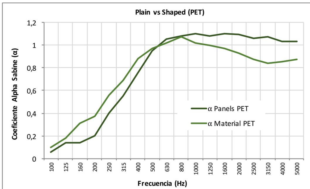
Figure 20. Absorption Coefficient PET Fiber Plain vs Shaped
