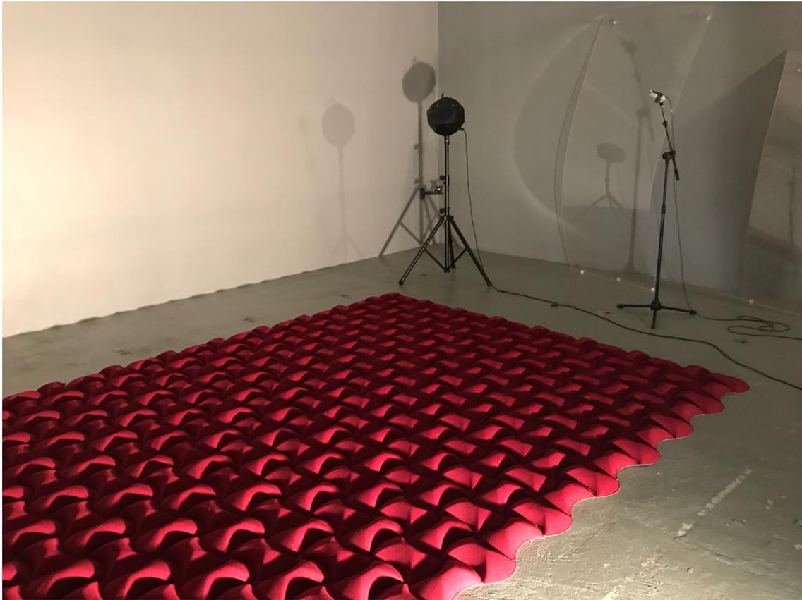
*Figure 15. Polyester Fiber + Fabric in Shaped fitting panels set up*
