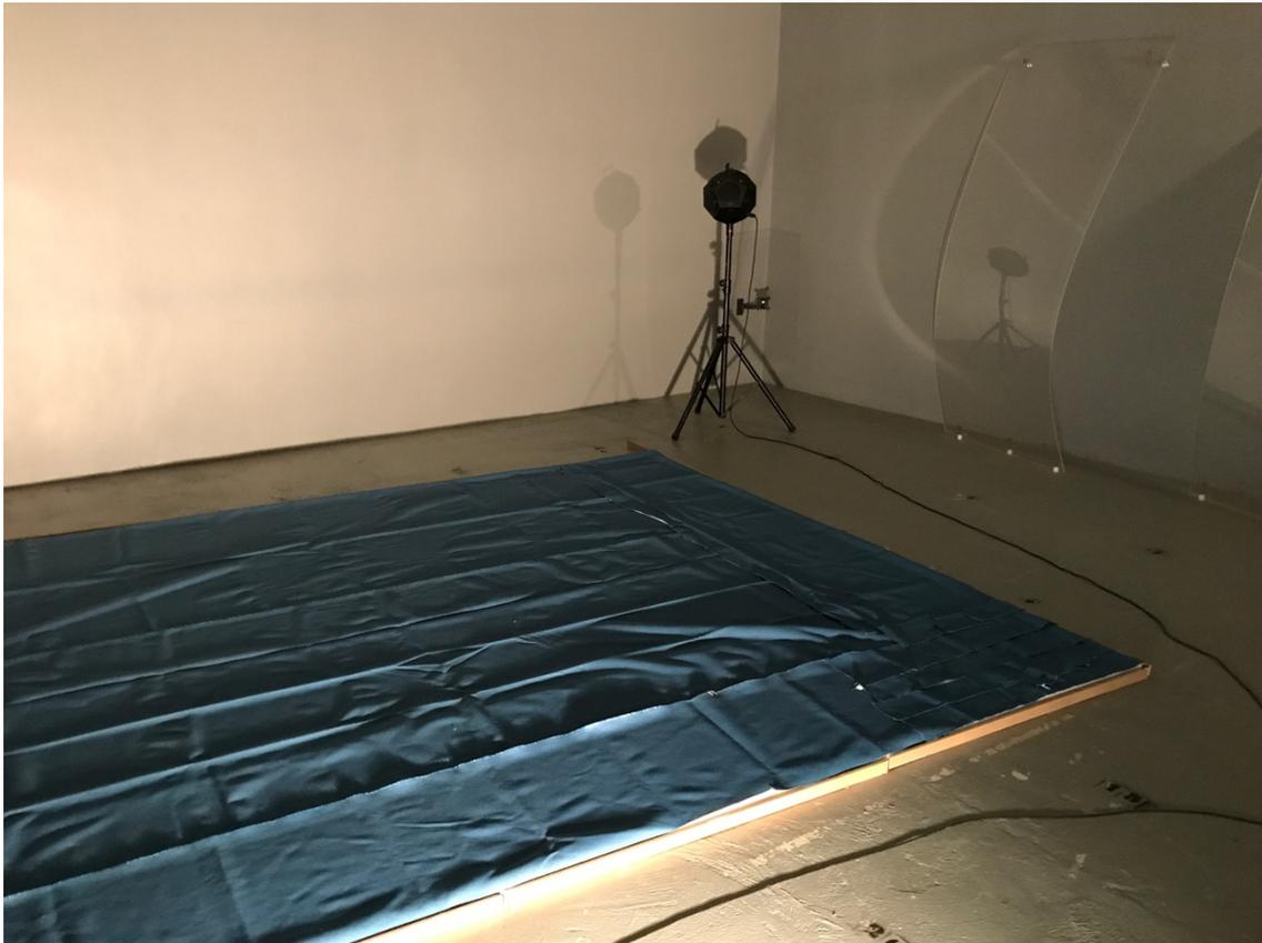
*Figure 13. Polyester Fiber + Fabric set up*
