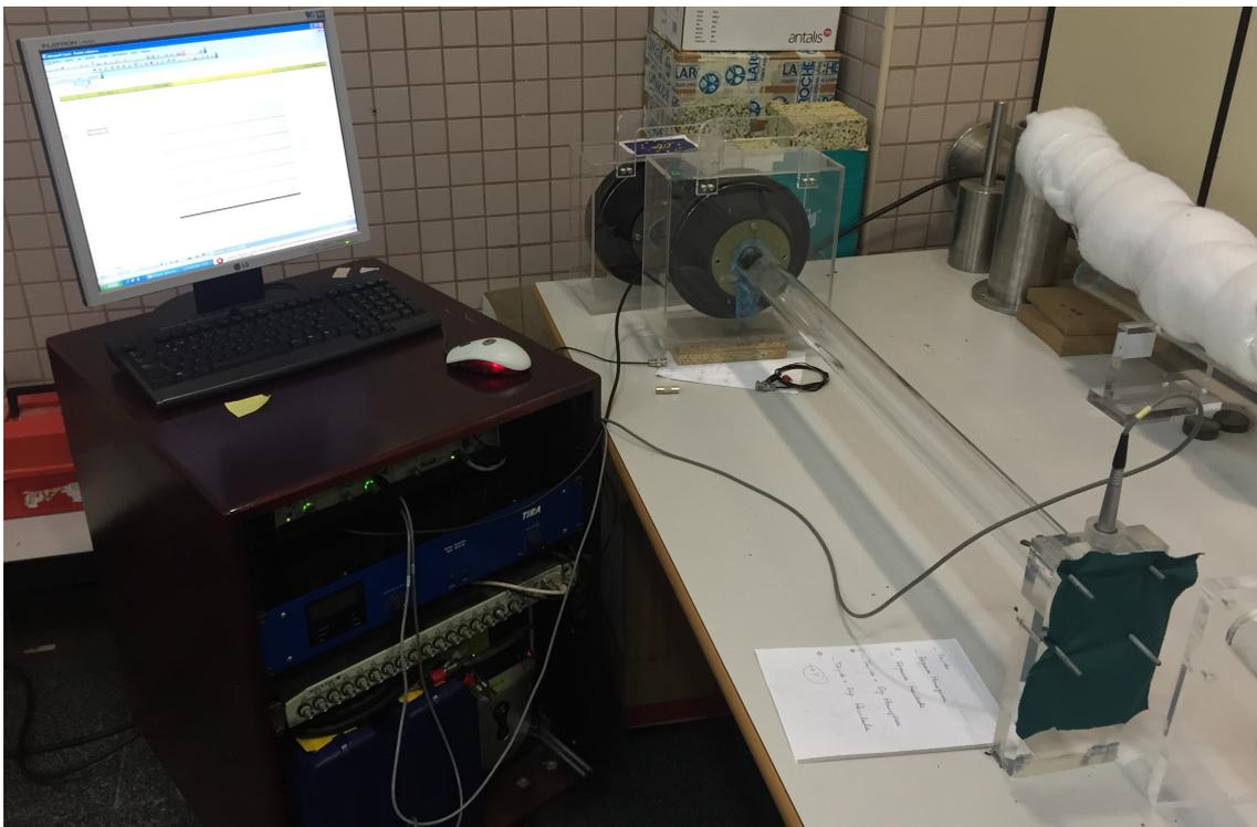
Figure 7. Airflow Resistance measurement Set-up
