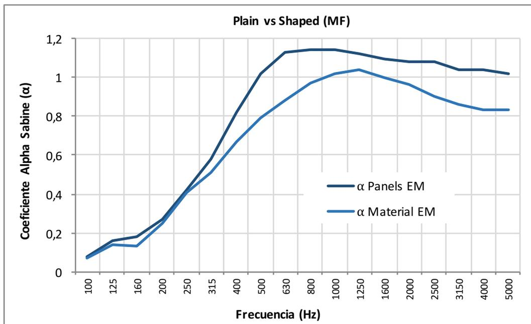
Figure 19. Absorption Coefficient Melamine Foam Plain vs Shaped
