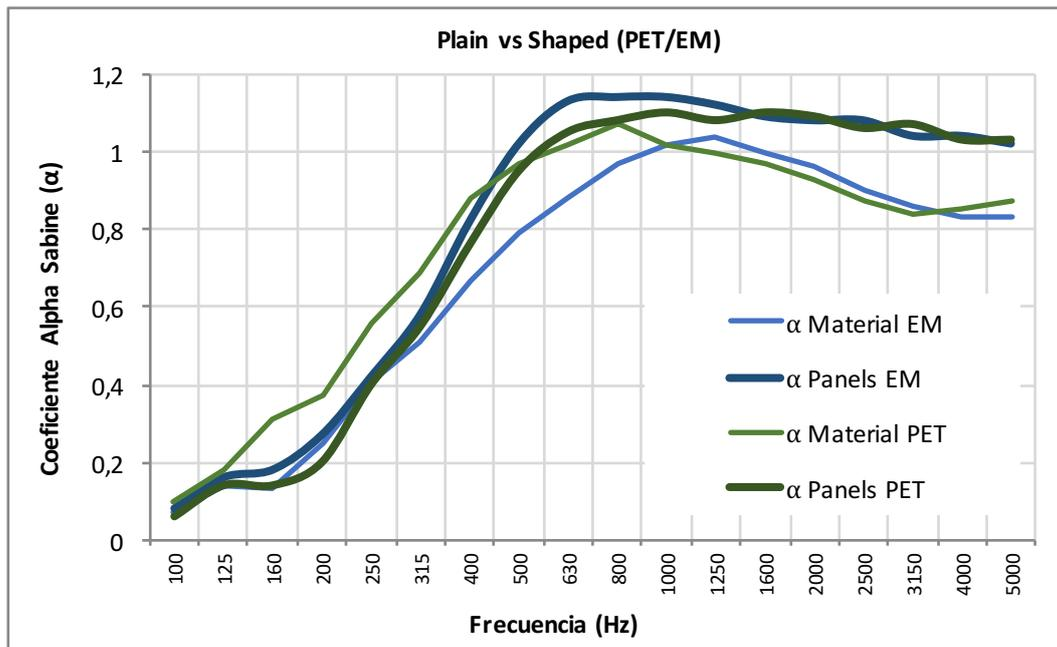
Figure 19. Absorption Coefficient Melamine Foam and PET Fiber Plain vs Shaped
