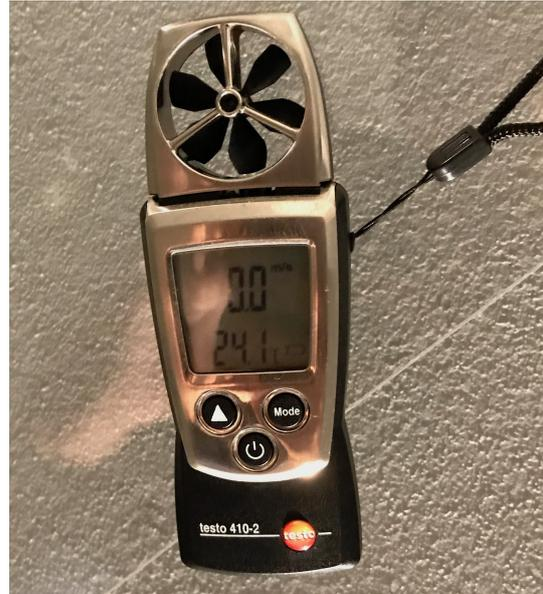
*b. Anemometer and Thermometer*
