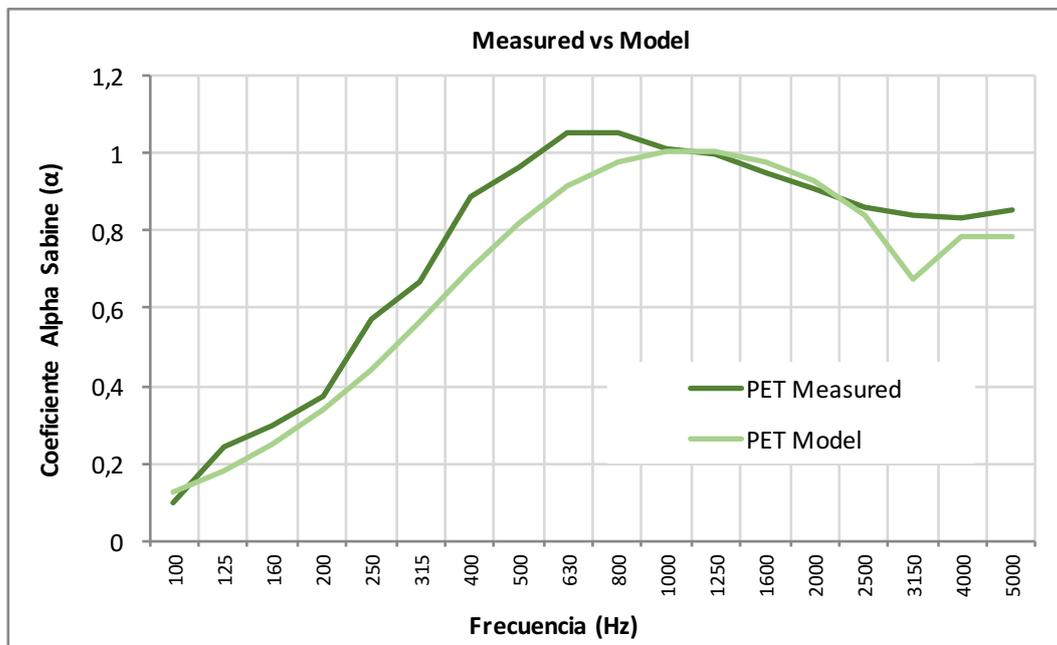
Figure 17. Absorption Coefficient PET Fiber
