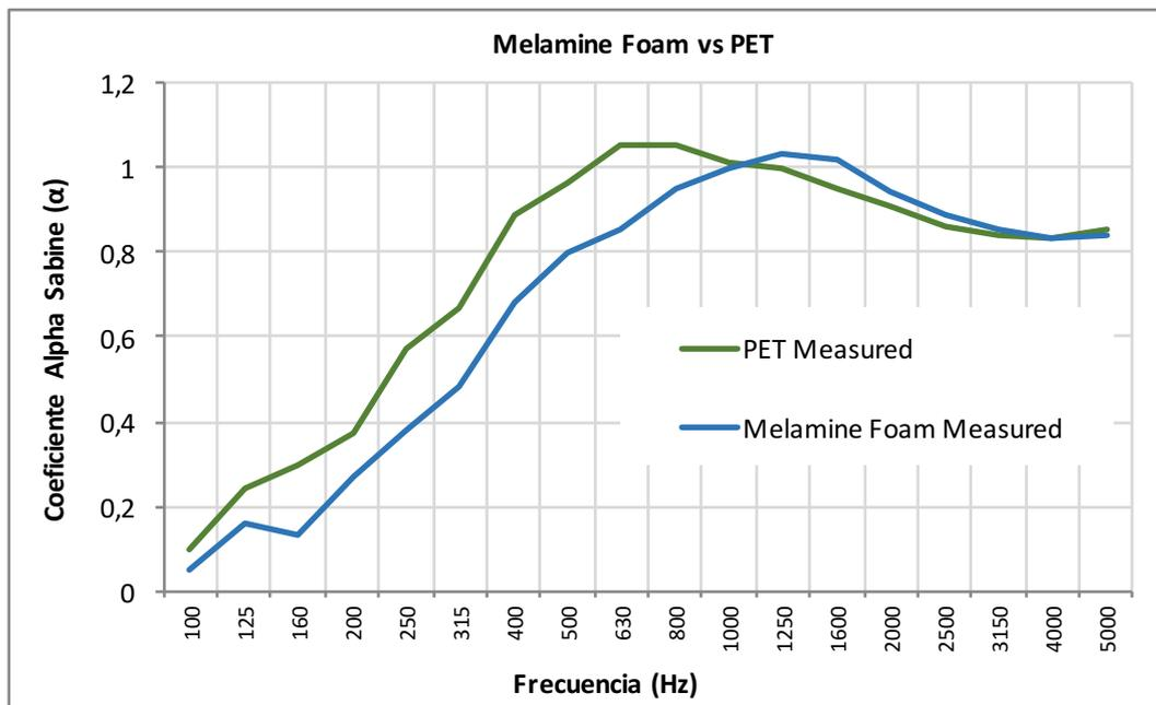
Figure 18. Absorption Coefficient Melamine Foam vs PET Fiber
