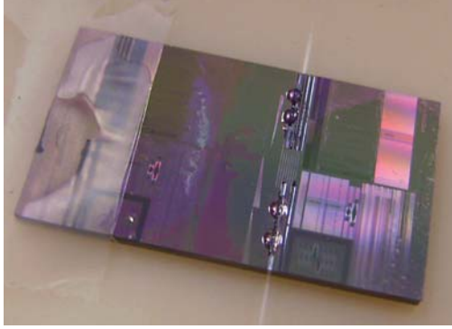
Figure 4.24: Photo of the V-groove sample after pigtailed.
