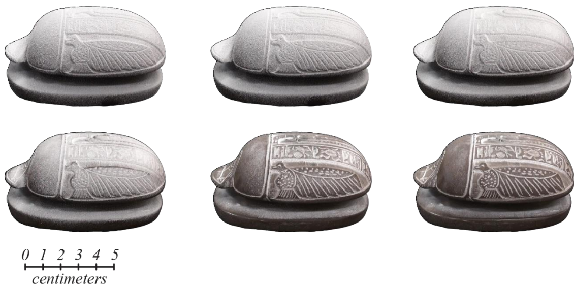
Figure 1: From left to right and top to bottom, the sublimation of cyclododecane applied on an artifact. Images are captured in 45 seconds intervals since the application of the spray (top-left picture). The process has been accelerated pointing a hair dryer towards the object. It is important to remark that, the white areas on the last picture are from the original artifact, since cyclododecane has completely sublimated.
