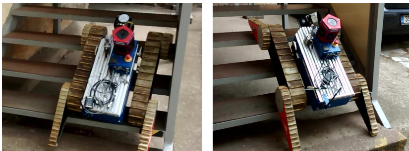
FIGURE 4.5: Examples of flippers stuck inbetween the steps of stairs.
