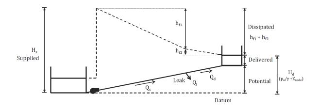
Fig. 1. Schematic representation of a simple system, including the main energy concepts.
