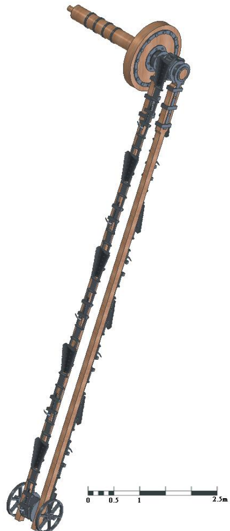
Figure 32: Assembly of the dredger elements.
