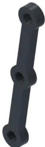
Figure 12: Axonometric view of the coupling of rocker arms and the piston axle.
