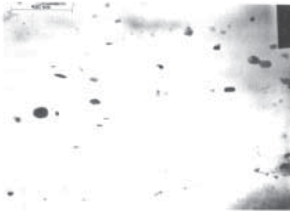
Fig 3 Precipitates in HAZ at a distance of 0.6 mm from the interface ( \times 21\ 500 ).
