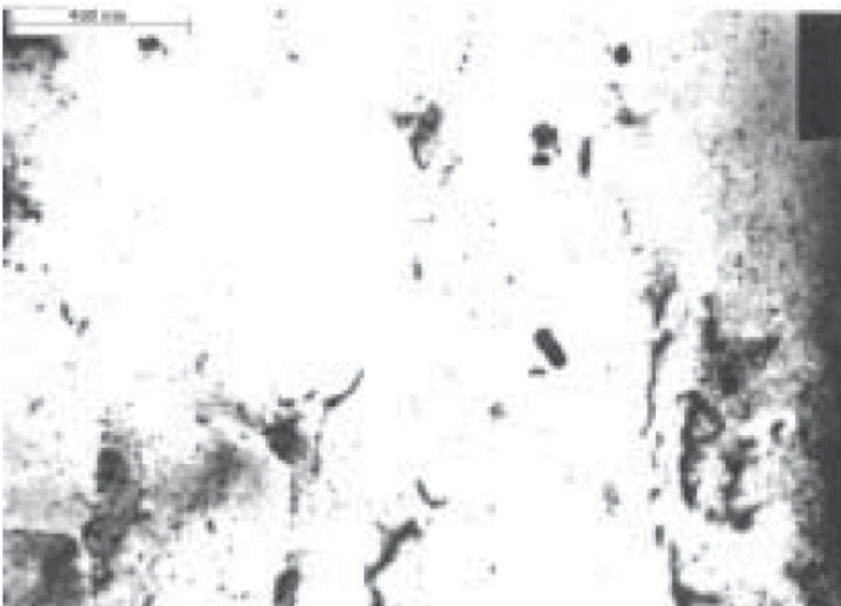
Fig 5 Precipitates in HAZ at a distance of 8.5 mm from the interface ( \times 21\ 500 ).
