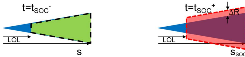
Figure 3.15. Schematic showing the simplified inert (left, t = t_{SOC^-} ) to reacting (right, t = t_{SOC^+} ) transition as described by the model.
