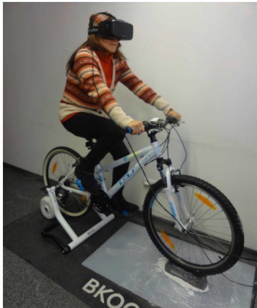
Figure 3.16: Locomotion interface (physical active condition)
