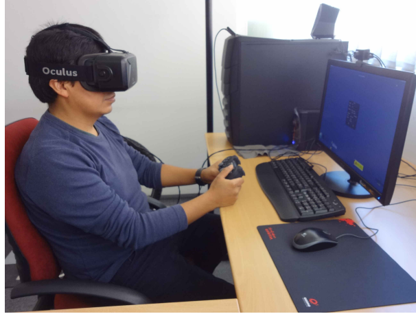
Figure 3.14: Stationary interface (physical inactive condition)
