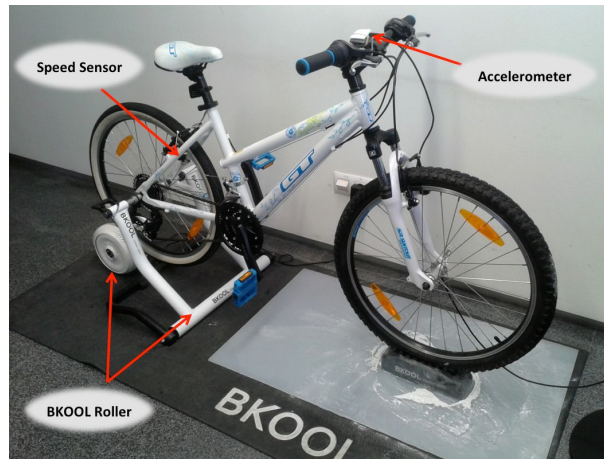
Figure 3.17: Bicycle on the Bkool roller and sensors.
