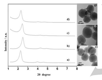
Figure 1. Left: powder X-ray patterns of the solids (a) MCM-41 as synthesized (b) calcined MCM-41, (c) solid S1 and (d) solid S1-mPh. Right: TEM images of (e) calcined MCM-41 sample, (f) solid S1 and (g) S1-mPh showing the typical hexagonal porosity of the MCM-41 mesoporous matrix.
