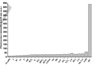
**Figure 2.** Fluorescence intensity at 610 nm of  $[Ru(bipy)_3]Cl_2$  dye released from **S1-mPh** (HEPES 10 mM at pH 7.5) after 6 h of adding 1 mM of selected anions, amino acids and oxidants.
