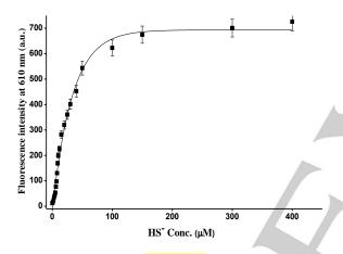
**Figure 3.** Calibration curve of [Ru(bipy)<sub>3</sub>]Cl<sub>2</sub> dye released from **S1-mPh** (HEPES 10 mM, pH 7.5) upon addition of increasing quantities of HS<sup>-</sup>.
