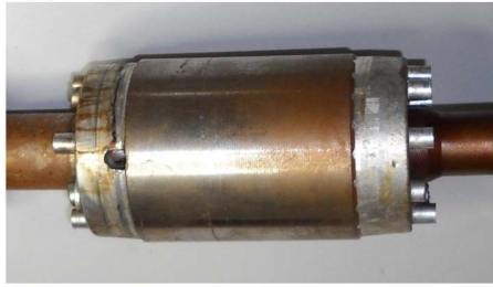
Fig. 5. Rotor featuring a broken bar.
