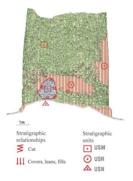
Fig. 3- Cala d'Oliva tower, stratigraphic analysis (Murru, 2014).
