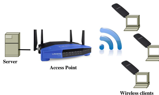
Fig. 1: Network deployment. Detail of the Video Streaming Server, the IEEE 802.11ac/n Access Point and Wireless clients.
