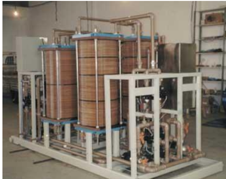
Figure 6. Electrodeialysis system for water demineralization (69).
