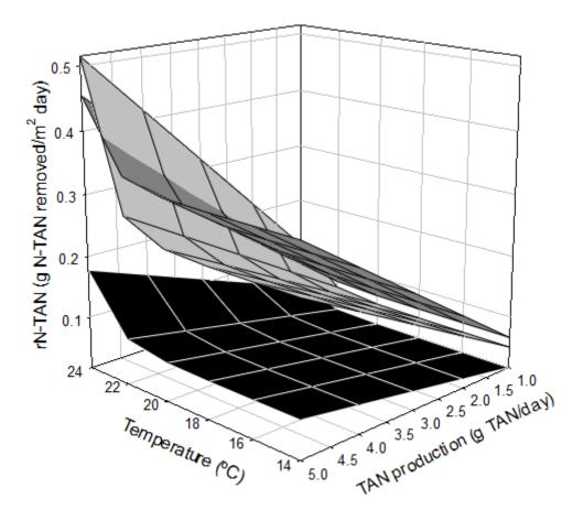
Figure 5. Three dimensional model showing quantitatively relations between N-TAN removal rates and the process parameters ammonia production and mean temperature for each one of the three filter media tested.
