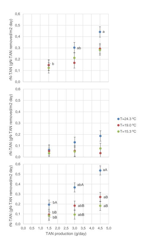
Figure 4. Mean N-TAN removal rates (±SEM: pooled standard error of the mean) achieved by biofilters classified by filter medium under fixed mean temperature and N-TAN influent concentration conditions. Small letters indicate statistical differences (p<0.05) on the N-TAN removal rates achieved depending on the N-TAN influent concentration whilst capital letters indicate significant differences on N-TAN removal rates achieved depending on the mean temperature.
