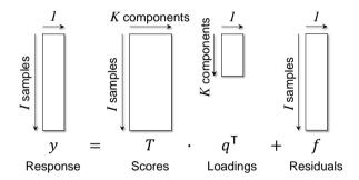
Fig. 3.18: Sketch of the matrices and vectors involved in the decomposition of the response vector by PLS.
