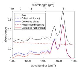
Fig. 3.9: Example of baseline correction methods.
