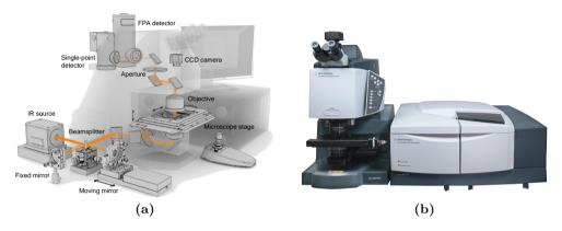
Fig. 2.9: (a) Schematic of main components in a common microspectrometer (spectrometer placed at left and microscope at right). Reproduced from [116] with permission by courtesy of SAGE publications Inc. (b) Photograph of a modern commercial microspectrometer (in this case, spectrometer placed at right and microscope at left). Reproduced from [117].
