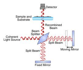
Fig. 2.4: Schematic diagram of a Michelson interferometer configured for FTIR spectroscopy. Adapted from [104].
