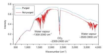
Fig. 2.13: Water vapour intensity spectrum. Intensity spectrum recorded when purging (blue) and not purging (red) the isolated sample compartment with dry air. Adapted from [138] with permission by courtesy of Macmillan Publishers Ltd.
