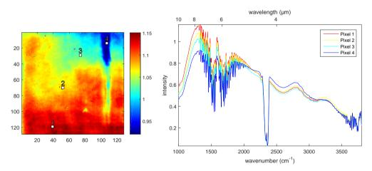
Fig. 2.17: Intensity reference spectra  $I_0(\tilde{\nu})$  of a FPA detector. Left: Pseudocolour image with its colourbar of the intensity values corresponding to a wavenumber  $\tilde{\nu} = 1300 \text{ cm}^{-1}$ . Right: Intensity reference spectra  $I_0(\tilde{\nu})$  of the pixels selected in the pseudocolour image.
