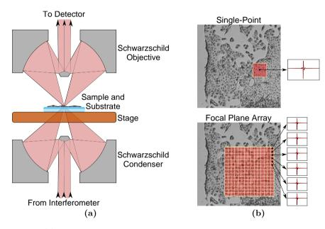
**Fig. 2.10:** (a) Sketch of the functioning of a Schwarzschild objective and condenser configured in transmission mode. (b) Sketch of the regions covered with a single-point (up) and a Focal Plane Array detector (down) in a cellular sample.
