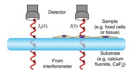
Fig. 2.6: Schematic of the acquisition of the reference background spectrum  $I_0(\tilde{\nu})$  and the intensity sample spectrum  $I(\tilde{\nu})$  in transmission measurements.
