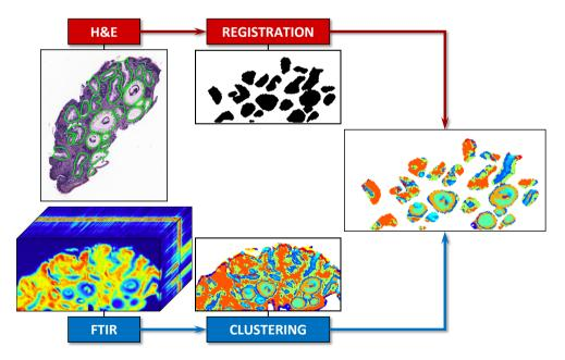
Fig. 4.11: Sketch of the fusion of spatial information obtained by registration and clustering.
