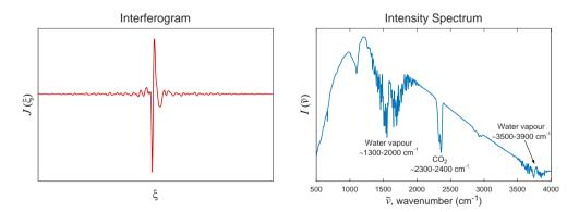
Fig. 2.5: Example of a recorded interferogram (left) and its associated intensity spectrum computed by applying the Fourier transform (right). These graphics correspond to a measurement with no sample. Some relevant absorption bands have been identified in the intensity spectrum. Adapted from [106].
