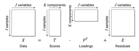
Fig. 3.13: Sketch of the matrices involved in the decomposition by PCA.
