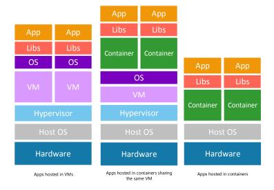
Figure 1: Virtual Machines and Containers possible architectural configurations.
