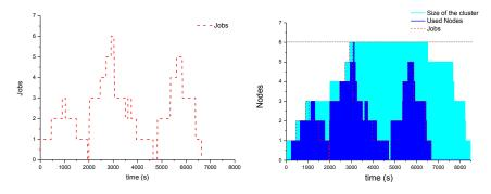
(a) Job pattern submission of the case study. (b) Execution on VMs (EC3 with idle time for scale-in set to 30 min).
