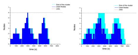
(c) Execution on containers (EC4Docker). (d) Execution on VMs (EC3 with idle time for scale-in set to 10 min).
