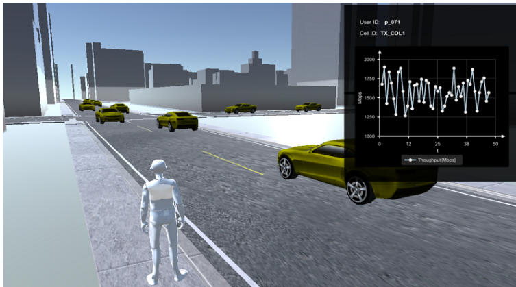
Figure 7.8: Example of a pedestrian user with a graph showing the evolution of the experienced data throughput in real time
