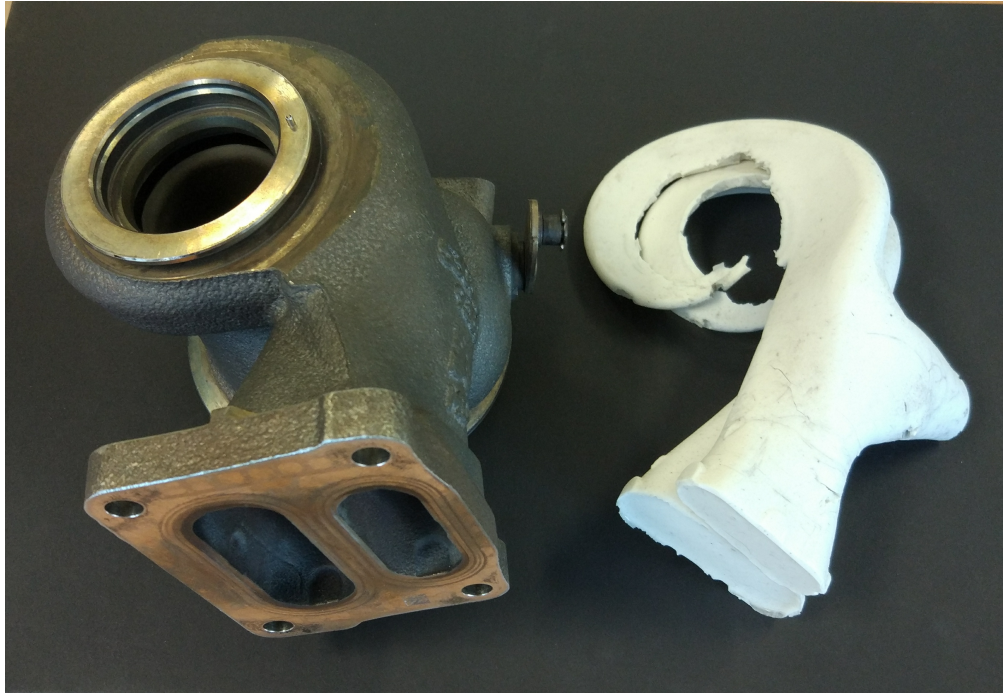
Figure 4.2: Turbocharger specimen and silicone mould.
