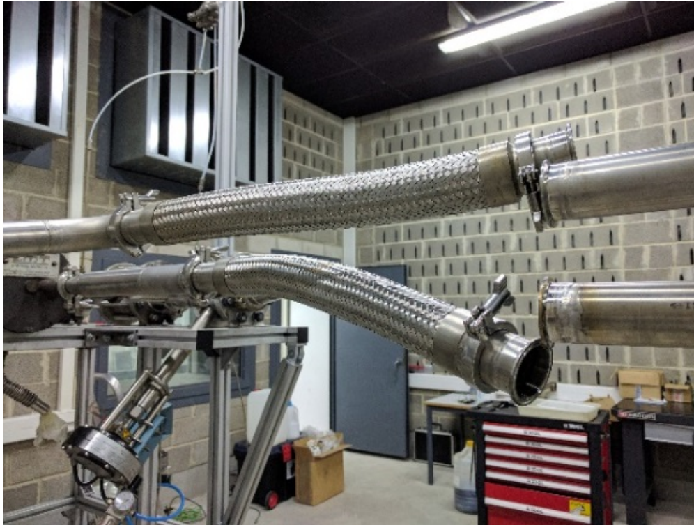
Figure 3.2: Flexible pipes for switching the pulsating branch.
