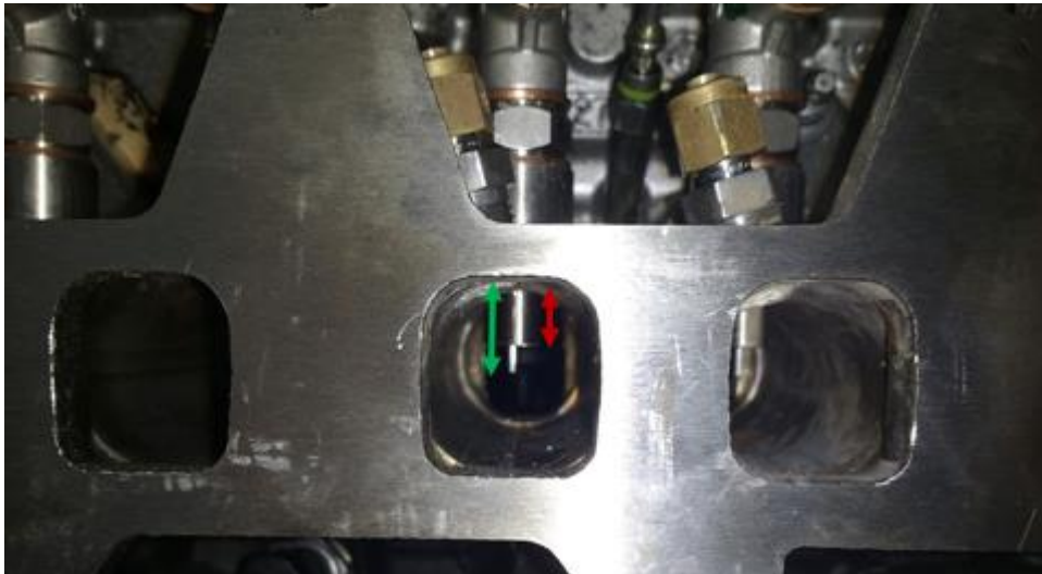
Figure 3.4. Detail of the sampling pipes in the intake runners.
