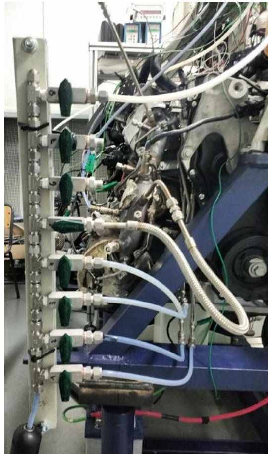
Figure 3.8. Rail and valves for exhaust gas measurement selection.
