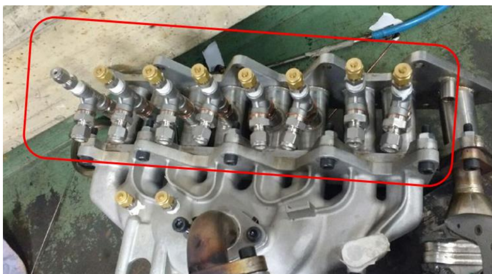
Figure 3.1. The eight probes installed in the intake to measure the gas composition in every pipe.
