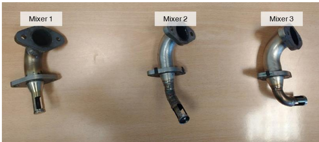
Figure 3.9. Devices that introduce and mix the EGR with the intake air in the manifold.
