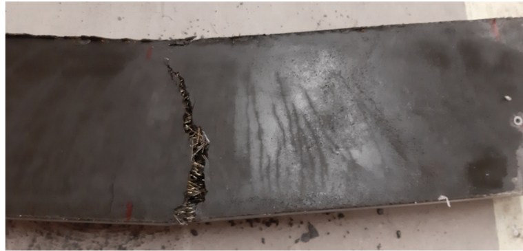
Figure 6.7 Collapsed short beam
