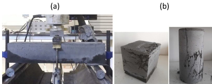
Figure 2.43 UHPFRC characterisation tests: (a) unnotched 3PBT and (b) compression test in (Yin et al. 2019a)
