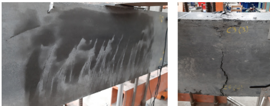
Figure 6.14 Microcracking (left) and collapse (right) of a long beam
