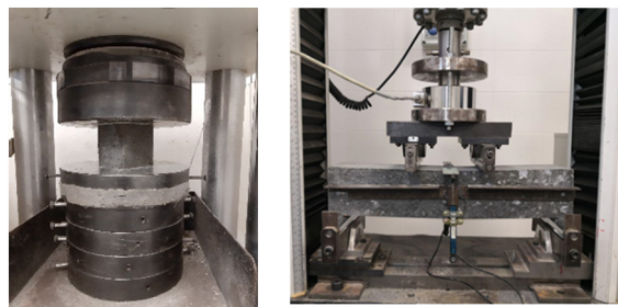
Figure 6.15 Compression test (left) and 4PBT (right)
