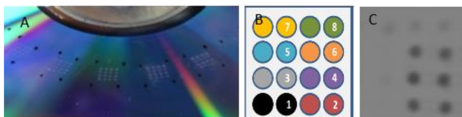
Figure 6.1.S2. A) Image of the array on the DVD surface; B) Lay-out of the antigens and controls printed on the DVD (Position 1: HSA, negative control, C(-); 2: human IgE, positive control, C(+); 3: Aztreonam-oyl antigen, negative control C(-); 4-7: antigen 1-4; 8: Reference antigen); C) Representative image of the array with specific antigens and controls printed on the DVD. Artificial human serum specific to PG was used.
