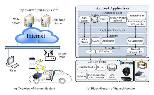
Figure 6.1: System architecture of DrivingStyles: Overview and block diagram architecture.
