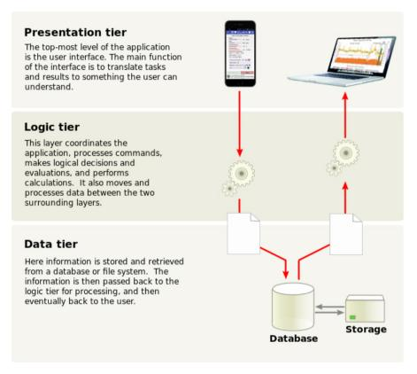
Figure 2.5: Overview of a three-tier application.
