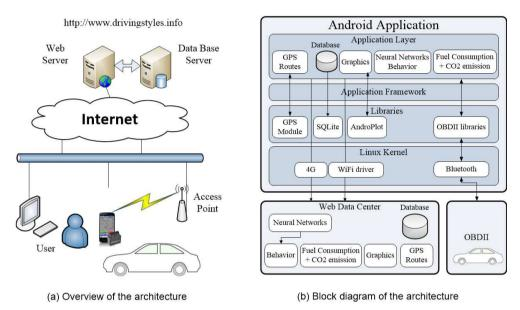
Figure 4.1: System architecture of DrivingStyles.
