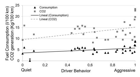
Figure 5.6: Chart of consumption and  $CO_2$  in relation to the driving behavior.
