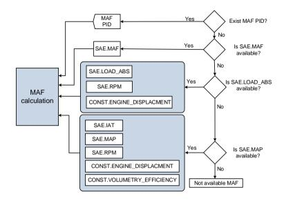
Figure 5.4: Scheme of the different MAF calculation possibilities regarding fuel consumption calculation.
