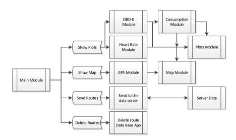
Figure 8.4: Android application's modules flow diagram.
