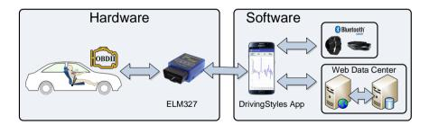
Figure 8.1: Overall hardware and software system architecture.
