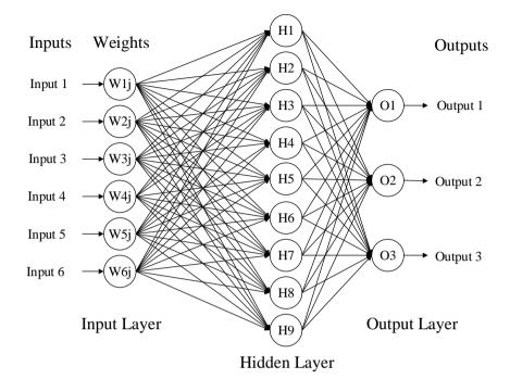
Figure 2.3: Schematic representation of a Three-layer Neural Networks.
