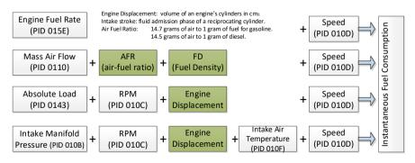
Figure 8.7: Methods used in Android app to calculate the instantaneous fuel consumption.
