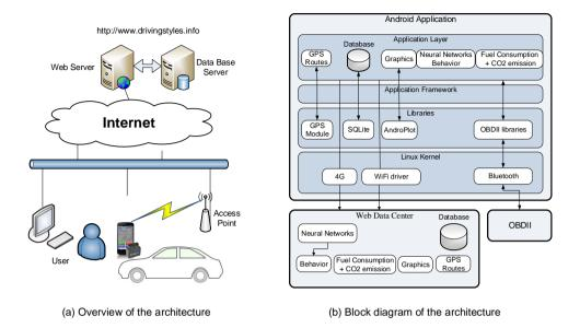
Figure 5.1: System Architecture of DrivingStyles.
