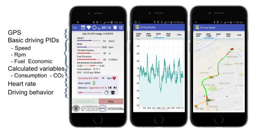
Figure 7.3: Snapshots of the main screen and the heart rate module for the Android application.
