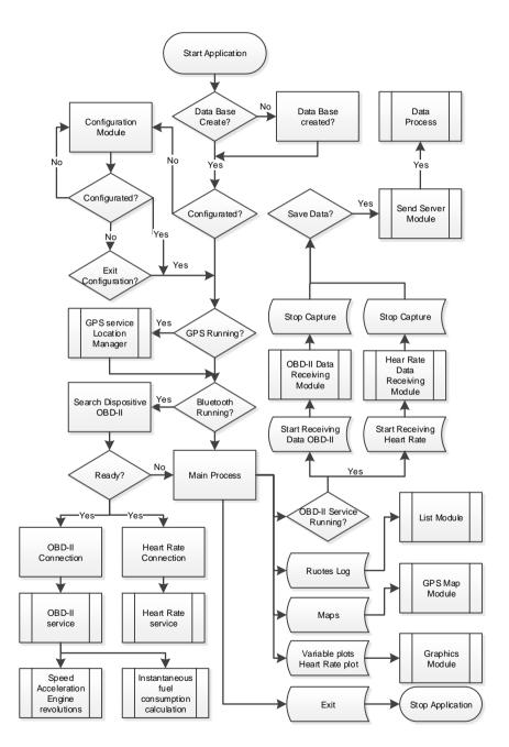
Figure 8.5: Android application's flow diagram.
