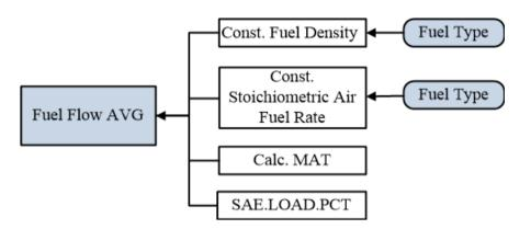
Figure 4.5: Outline of the calculation of the Fuel Flow average.
