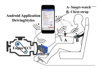
Figure 7.2: On Board schema components of DrivingStyles instrumentation.
