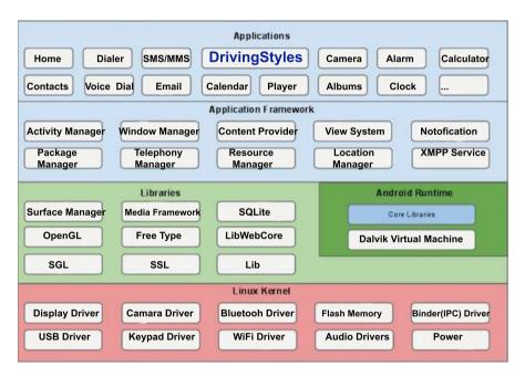
Figure 2.4: Android operating system stack of software components.
