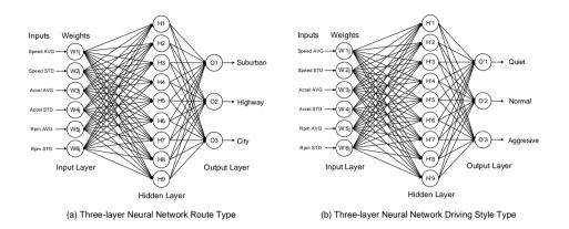
Figure 5.5: Schematic representation of the Three-layer Neural Networks used in the DrivingStyles Architecture.
