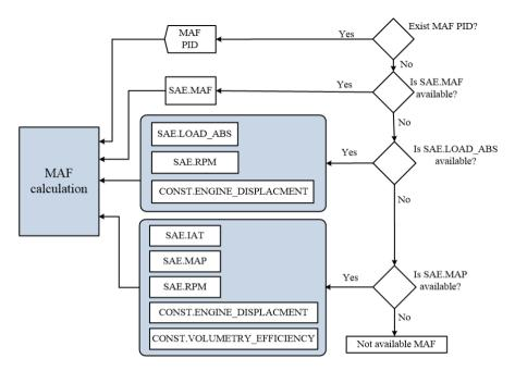
Figure 4.4: Scheme of the different possibilities of MAF calculation.
