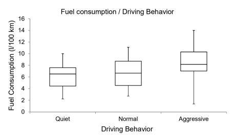
Figure 5.7: Box and whisker plot of Fuel Consumption/Driving Behavior.
