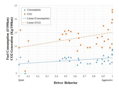
Figure 4.6: Chart of consumption and  $CO_2$  in relation to the driving behavior.
