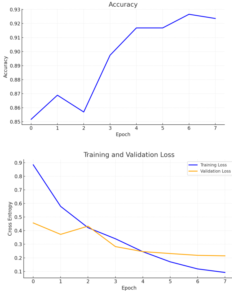
Figure 30 ResNet-18 accuracy & training & validation loss
